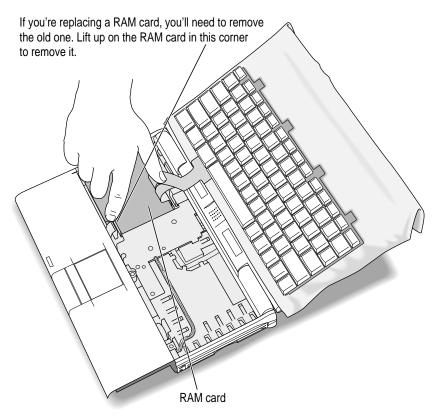
Be careful not to touch other parts of the computer's interior when lifting the card. Some parts may be hot if the battery has been charging or the computer has recently been used.
